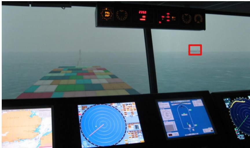
Figure 4-8. Indication of dangerous target projected as a red box on the bridge window.
